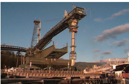
Running a terminal such as PCT, means overseeing large machinery such as the shiploader, which stands 40 meters tall.
