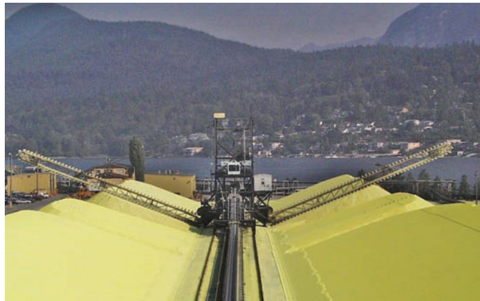
At PCT, sulphur is stored in large piles made by the 27-metre high Stakrake.
