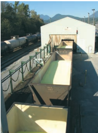
Trains carrying sulphur arrive at PCT, where the Rotary Car Dumper unloads the sulphur from the railcars onto conveyor belts.
